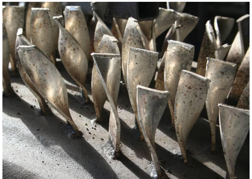
Heat sinks on the outside of the aluminium mould
