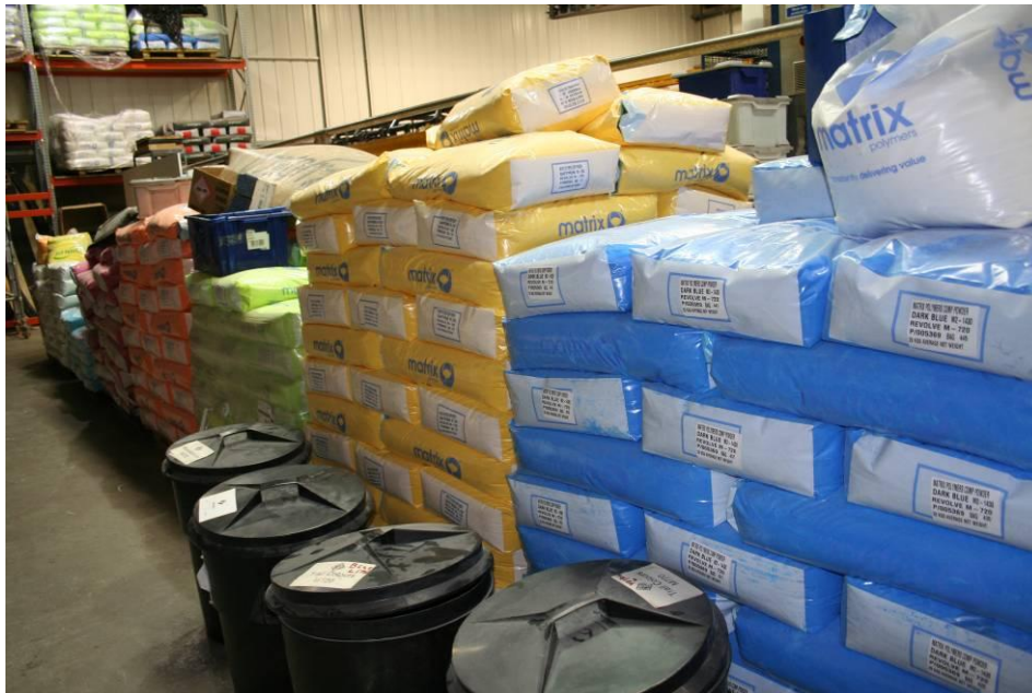
Different coloured plastic powders ready to be used for manufacturing new boats
