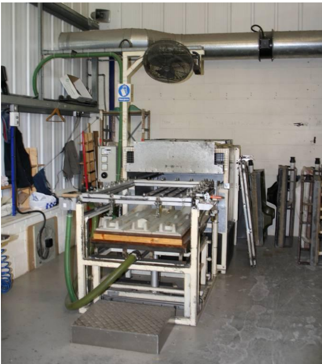
Seats are vacuum formed (left) and waste offcuts are collected for reprocessing (right)
