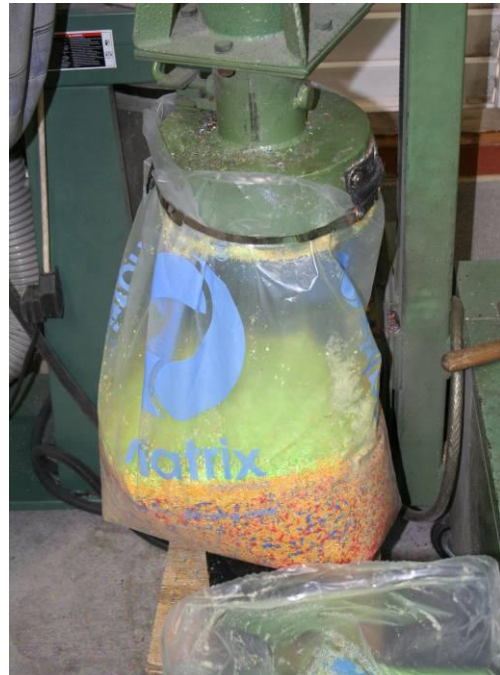
Plastic offcuts from the manufacturing process are collected and shredded on site
