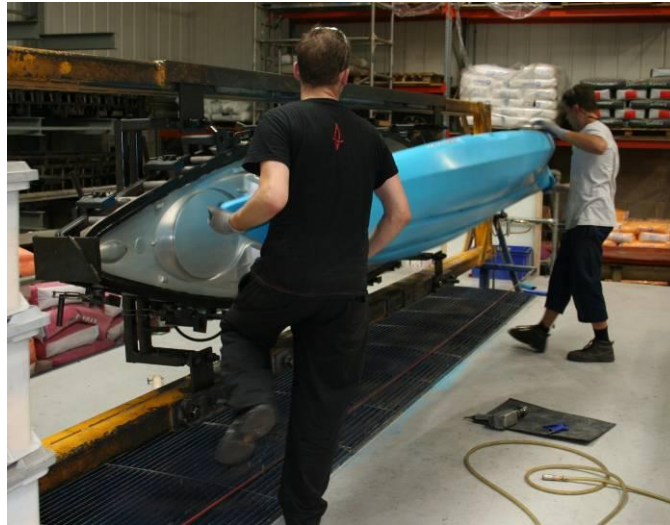
Removing the new kayak from the mould
