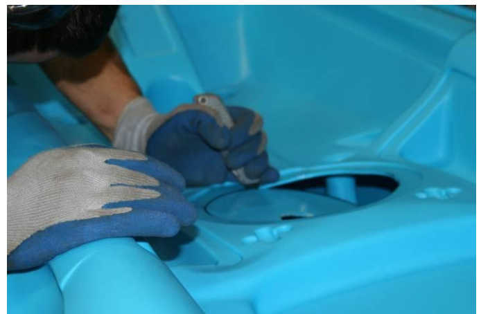
Offcuts are generated from cutting out plastic for hatches
