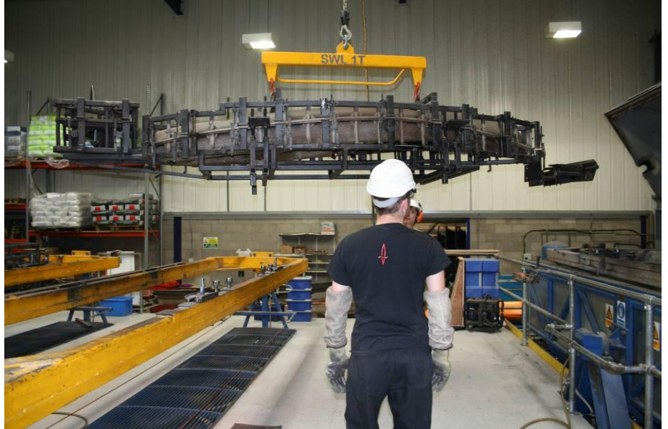
The new kayak is removed from the oven and placed on a rotating table to cool
