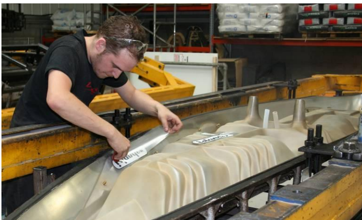
Careful application of graphics to the mould can help to minimise manufacturing defects
