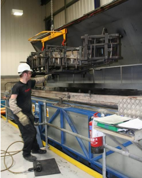
The new kayak is removed from the oven and placed on a rotating table to cool
