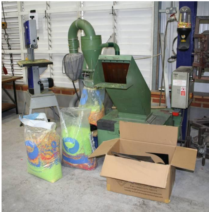
Plastic offcuts from the manufacturing process are collected and shredded on site
